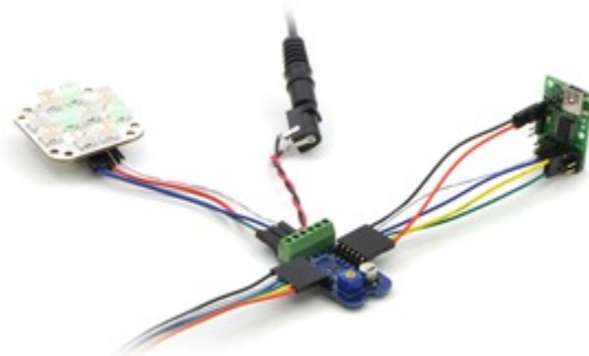
Connecting the Micro Maestro to a chain of ShiftBars. A single 12V supply powers all of the devices.
